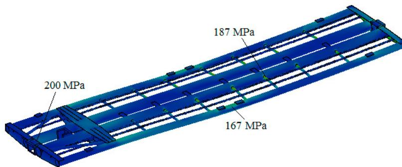
Fig. 3. The stressed state of the section of the articulated flat wagon (side view).
