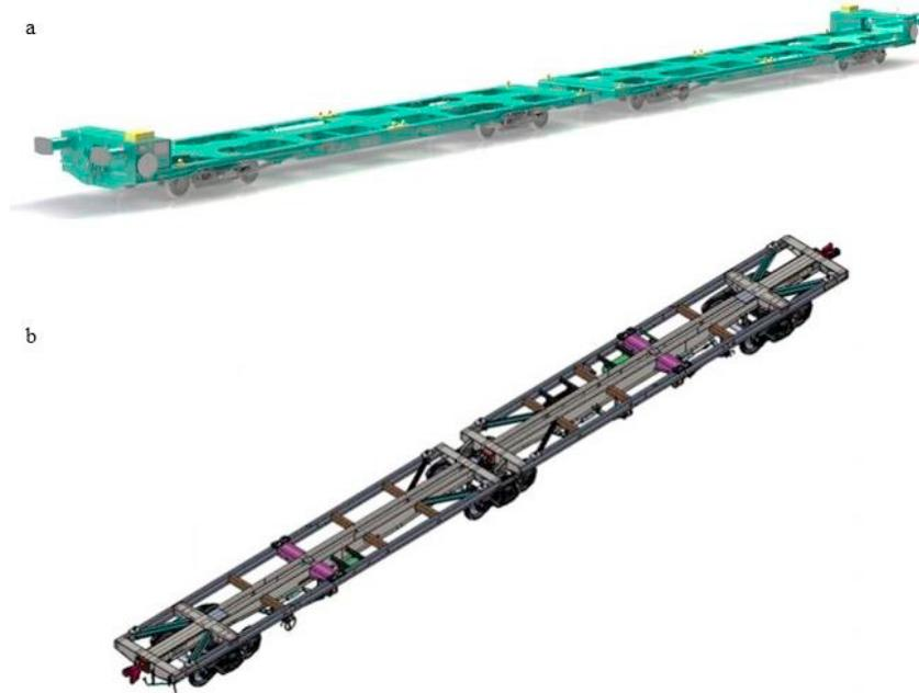
Fig. 1. Flat wagons of articulated type: (a) model FLA 2x40'; (b) model 13-9894.
