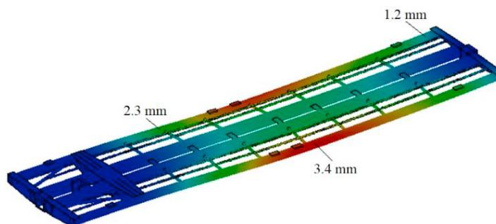
Fig. 5. Displacement in the nodes of a section of an articulated flat wagon.
