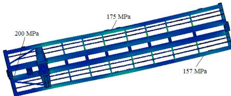
Fig. 4. The stressed state of the section of the articulated flat wagon (bottom view).
