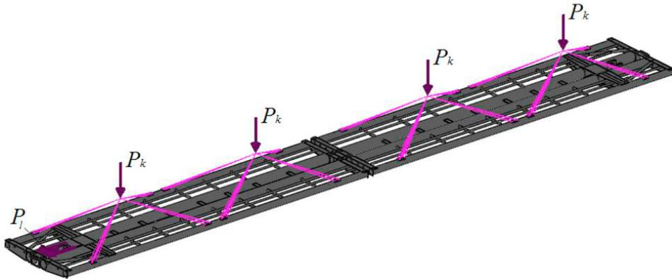
Fig. 2. Analytical model of the bearing structure of the articulated flat wagon made from round pipes.
