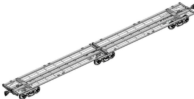
Fig. 2. Articulated flat wagon made from pipes of a circular cross section.
