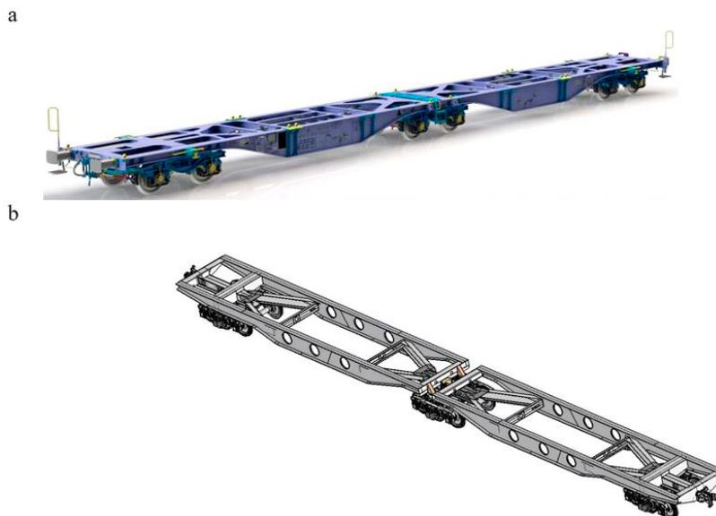
Fig. 1. Flat wagons of articulated type: (a) Sggmrss\_90; (b) model 13-1839.
