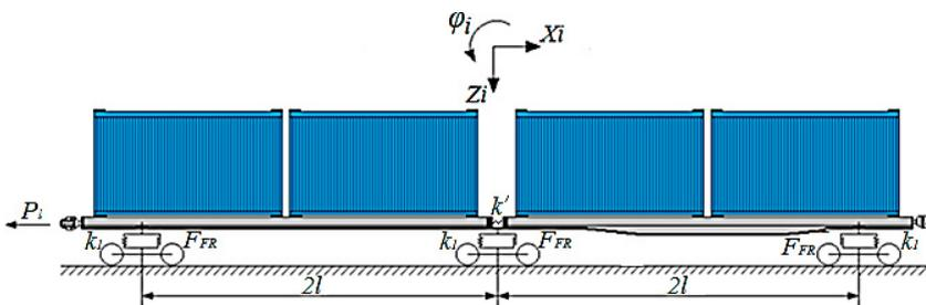
Fig. 3. The scheme of action of longitudinal force on a flat wagon of articulated type with containers placed.
