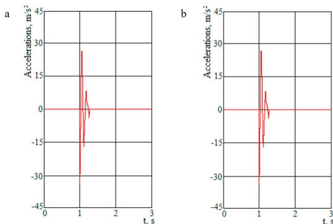
Fig. 4. Accelerations which act on the bearing structure of articulated flat wagon under I rated conditions (tension – jump): a) first section of flat wagon from the side of longitudinal force action; b) second section of flat wagon from the side of longitudinal force action.
